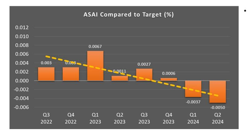
ASAI is calculated by dividing the total hours in which service is available to customers by the total hours that service is demanded by customers
