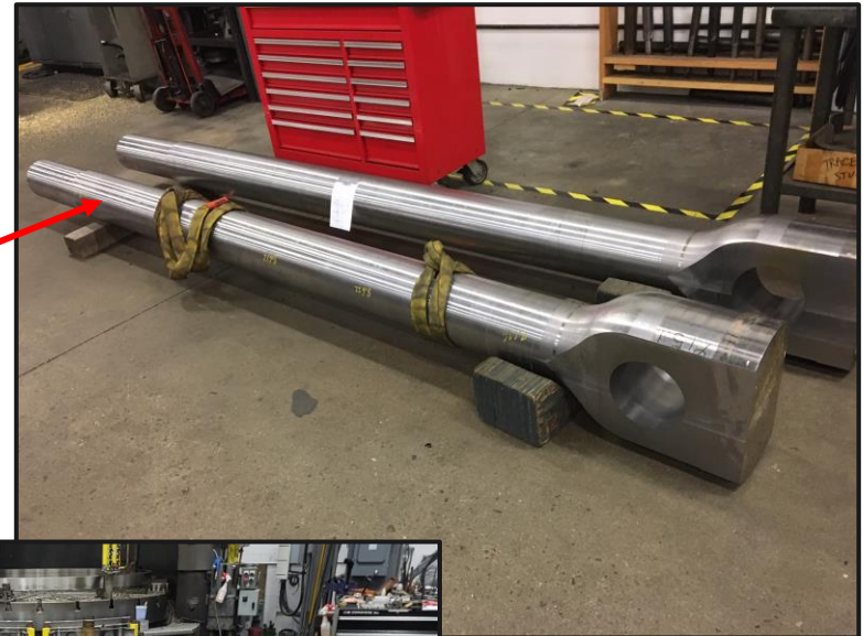
New Link Rods (Machined)
