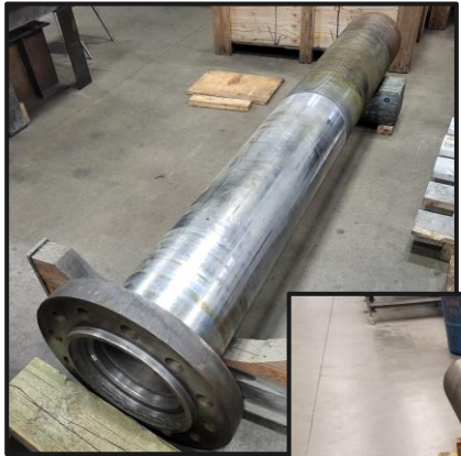
Worn Outer Piston Rod
