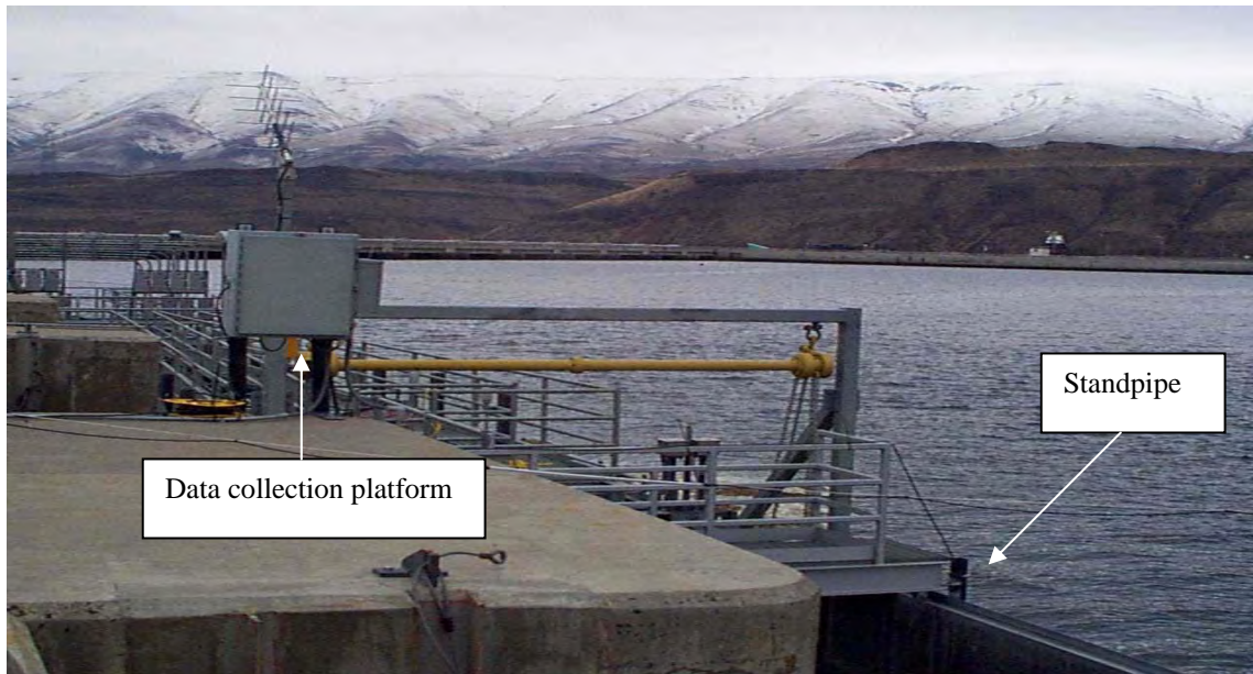
Figure 5 Photograph of Wanapum Dam forebay water quality fixed site monitoring station, Priest Rapids Project, mid-Columbia River.
