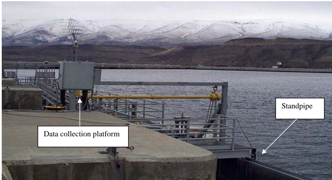
Figure 5 Photograph of Wanapum Dam forebay water quality fixed-site monitoring station (FSM station), Priest Rapids Project, mid-Columbia River.
